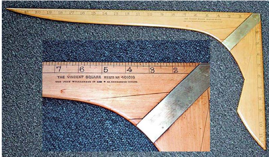
Fig. 12: 23 x 12 x 1/4 inch Curved "Vincent" Square in boxwood with a brass strap
